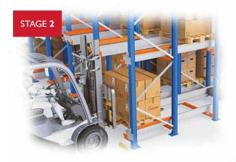
Then, the pallet is brought to the entrance of the lane using a forklift and placed on the load profiles.
