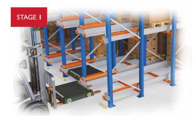
The shuttle is placed on the lane where it is to be operated by a forklift.
