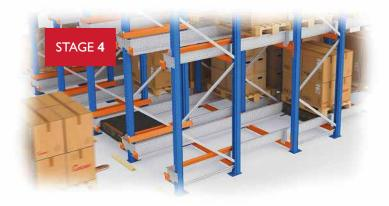
In the last stage, the shuttle performs the same action at the beginning of the lane where it picks up the next pallet and repeats the operation until the lane is full.
