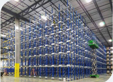
These are high-rise palletized load storage systems whose load units are handled by satellite shuttle cars.
